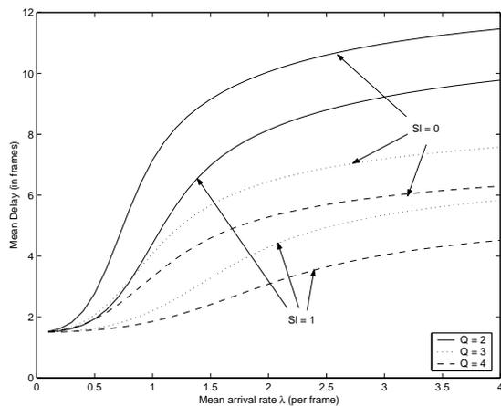
**Figure 8.15:** *The impact of  $S_l$  and  $Q$  on the mean delay*
