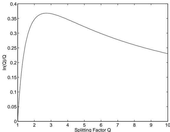
**Figure 1.1:** Influence of the Splitting Factor on the Maximum Stable Throughput for the Basic  $Q$ -ary CTM Algorithm
