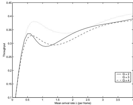
**Figure 8.14:** *The impact of  $Q$  on the throughput results for  $N_p = 20$*
