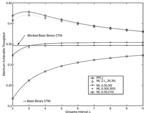
**Figure 5.1:** The impact of  $\Delta$  on the maximum stable throughput (basic)
