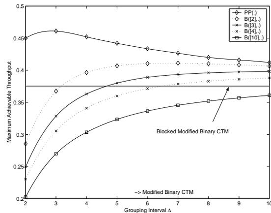
**Figure 5.6:** *The impact of  $\Delta$  on the maximum stable throughput (modified)*
