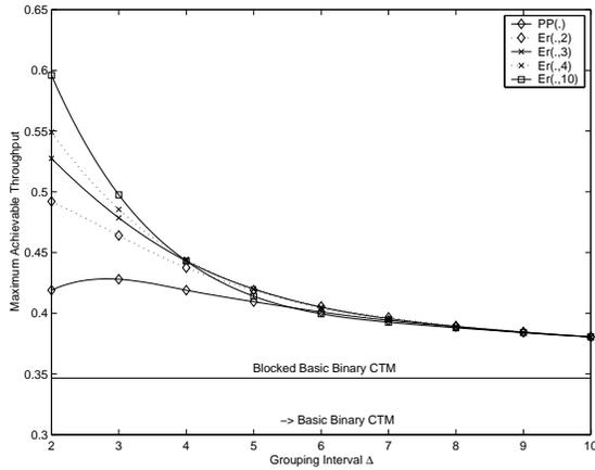
**Figure 5.3:** *The impact of  $\Delta$  on the maximum stable throughput (basic)*
