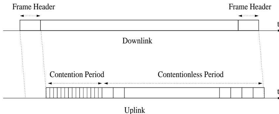
**Figure 6.2:** *Frame Structure*
