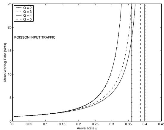
**Figure 4.2:** *The mean delay of the basic CTM algorithm with free access under Poisson input*
