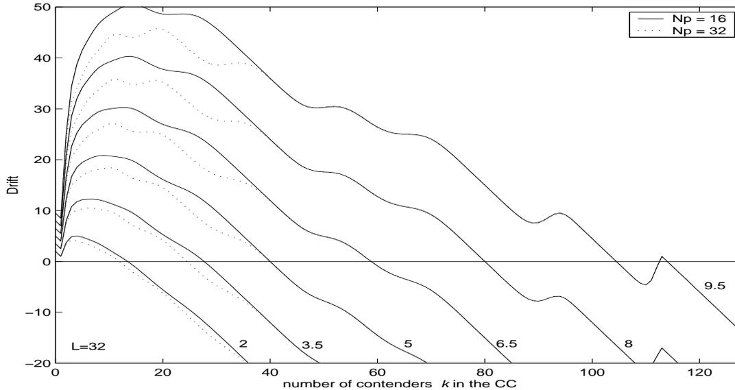
**Figure 8.26:** *Stability points for Poissonian input traffic*
