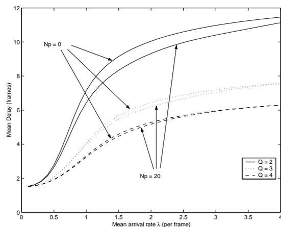
**Figure 8.11:** *The impact of  $Q$  and  $N_p$  on the mean delay*
