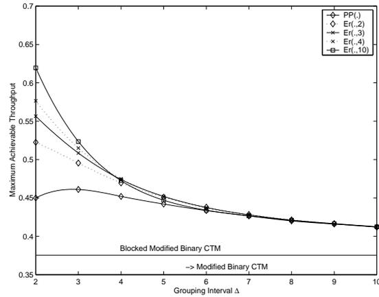
**Figure 5.4:** *The impact of  $\Delta$  on the maximum stable throughput (modified)*
