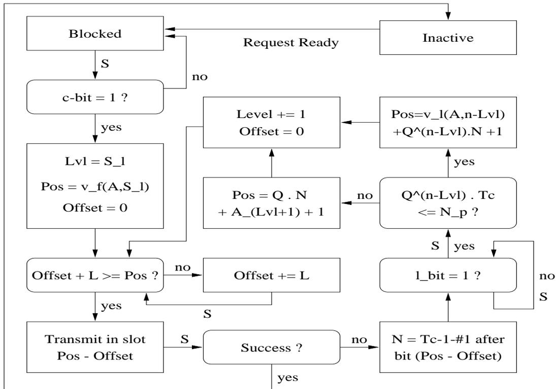
**Figure 6.5:** The Flow Chart of an MS ( $A = \text{MAC address of the MS}$ )
