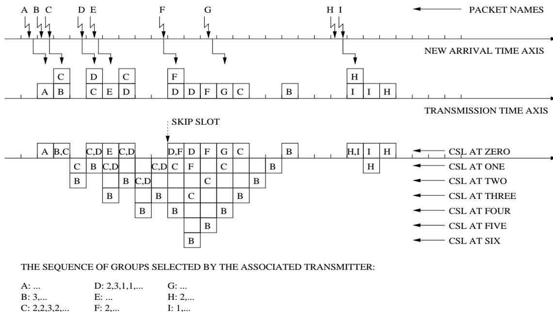
**Figure 4.1:** Example of the Transmission Process: CSL = Current Stack Level
