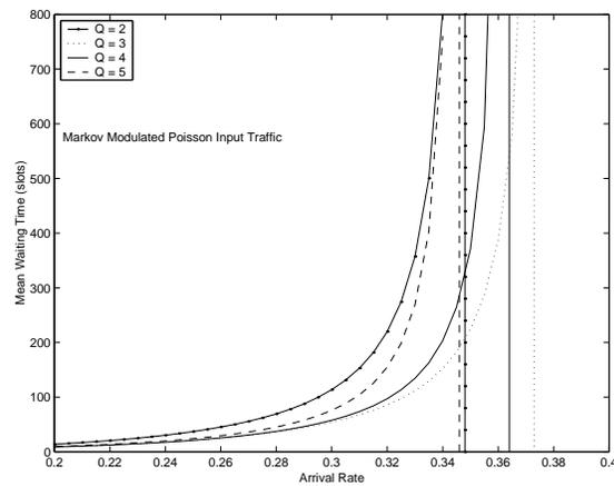
**Figure 4.5:** The mean delay of the basic CTM algorithm with free access under  $M(\lambda_1, 0, 30, 30)$  traffic
