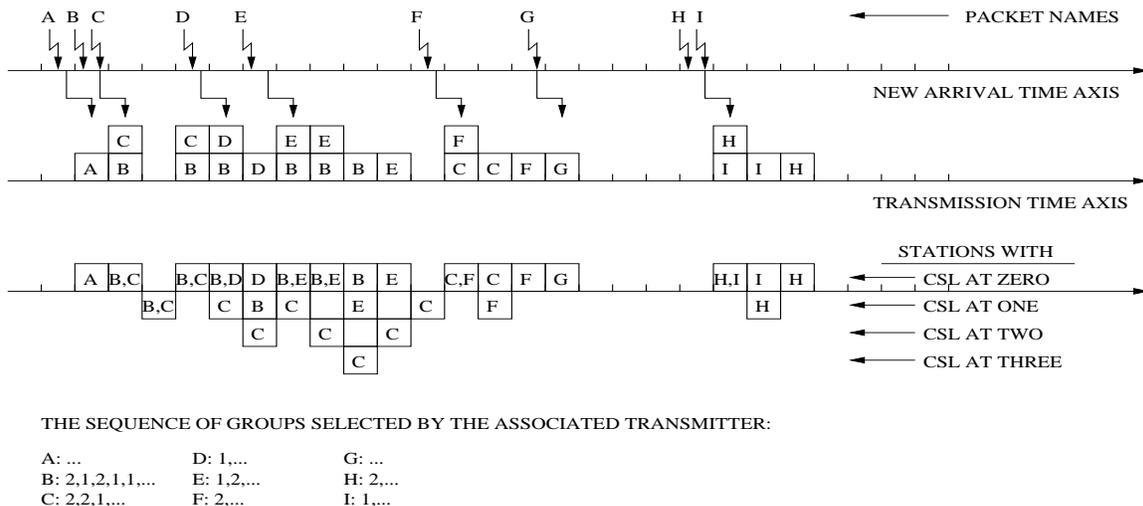
Figure 3.2: Example of the Transmission Process: CSL = Current Stack Level
