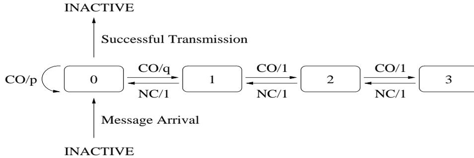
**Figure 3.1:** State Diagram:  $CO$  = collision,  $NC$  = no collision
