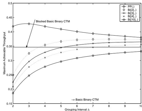
**Figure 5.5:** *The impact of  $\Delta$  on the maximum stable throughput (basic)*
