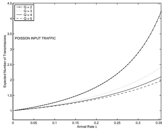
**Figure 4.3:** *The expected number of transmissions of the basic CTM algorithm under Poisson input*
