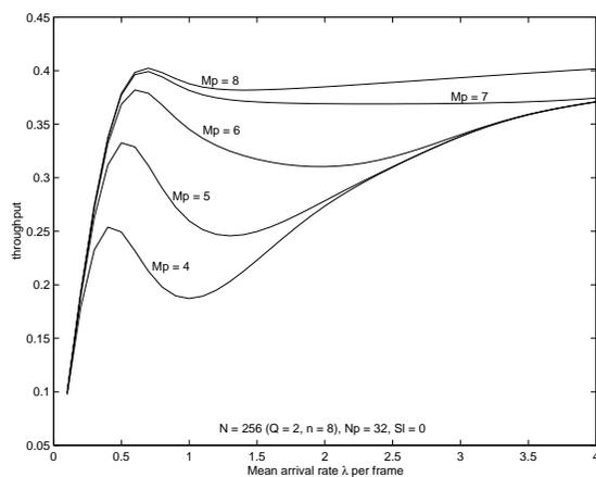
**Figure 8.18:** *The impact of  $M_p$  on the throughput*
