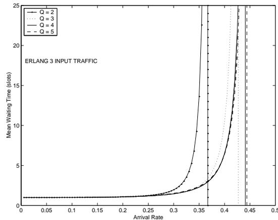
**Figure 4.4:** The mean delay of the basic CTM algorithm with free access under  $ER(\lambda_e, 3)$  input
