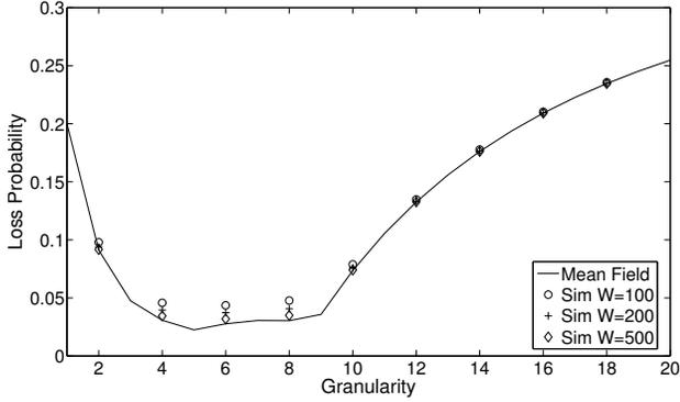
(b) *minimum gap* policyFigure 3. Mean field model vs. simulation for a switch with  $N = 5$ ,  $\rho = 0.8$ ,  $\sigma = 10$ , packet size equal to 10 and geometric IATs
