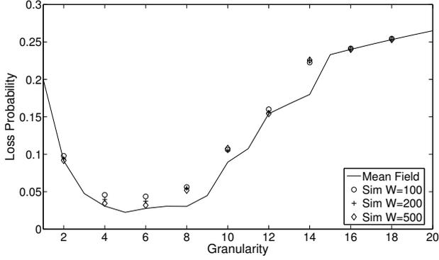
(a) *minimum horizon* policy
