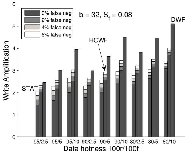
Figure 5: The effect of false negatives on the write amplification of the STAT, HCWF and DWF approach under a Rosenblum workload model for various choices of  $r$  and  $f$ , with  $b = 32$  pages per block and a spare factor  $S_f = 0.08$ .
