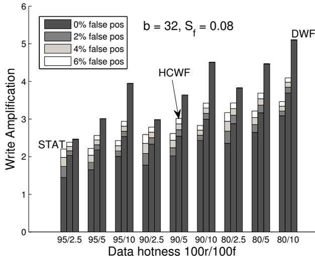
Figure 4: The effect of false positives on the write amplification of the STAT, HCWF and DWF approach under a Rosenblum workload model for various choices of  $r$  and  $f$ , with  $b = 32$  pages per block and a spare factor  $S_f = 0.08$ .
