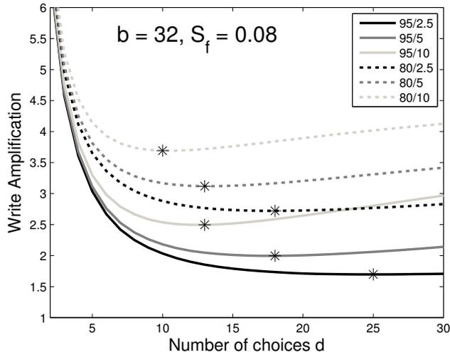
Figure 1: The impact of the number of choices  $d$  on the write amplification for the HCWF approach under a Rosenblum workload model for various choices of  $r$  and  $f$ , with  $b = 32$  pages per block and a spare factor  $S_f = 0.08$ .
