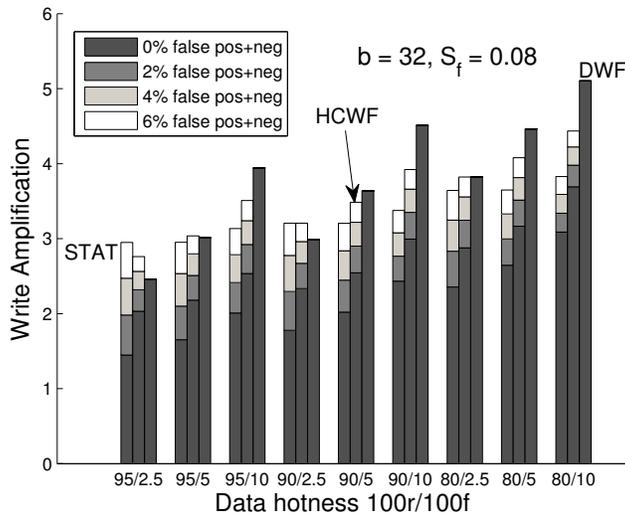
Figure 6: The effect of false positives and negatives on the write amplification of the STAT, HCWF and DWF approach under a Rosenblum workload model for various choices of  $r$  and  $f$ , with  $b = 32$  pages per block and a spare factor  $S_f = 0.08$ .
