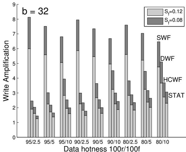
Figure 3: Write amplification of the SWF, DWF, HCWF and STAT approach under a Rosenblum workload model for various choices of  $r$  and  $f$ , with  $b = 32$  pages per block and a spare factor  $S_f = 0.12$  and  $0.08$ .
