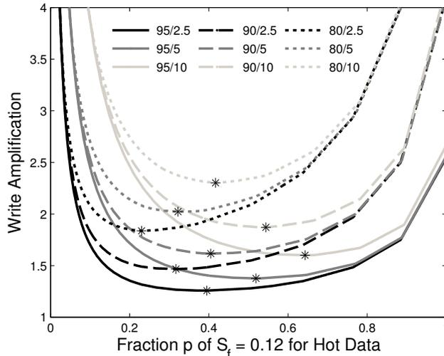
Figure 2: Impact of the fraction  $p$  assigned to the hot partition on the write amplification of the STAT approach in an SSD with  $b = 32$  pages per block and a spare factor  $S_f = 0.12$ .
