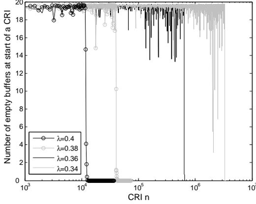
Figure 2. Simulation of the number of empty queues for  $J = 20$  users,  $\text{SNR} = \infty$  dB and various  $\lambda$  values (with  $\lambda_{max} = 0.31868$ ) for SICTA/FS.
