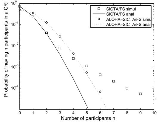
Figure 6. Analytical vs simulation results for the number of participants in a CRI with SNR =  $\infty$  dB,  $J = 20$ .  $\lambda$  equals 0.3 for SICTA/FS and 0.5 for ALOHA-SICTA/FS (with  $p_A = 1.5/J$ )
