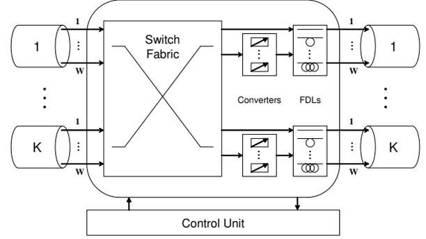
Figure 1. Optical switch with  $K$  input/output ports,  $W$  wavelengths, converters and FDLs
