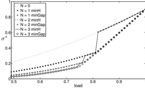
Figure 6. Comparison of policies for a switch with  $D = 10$ , geometric arrivals and packet size uniformly distributed between 5 and 15
