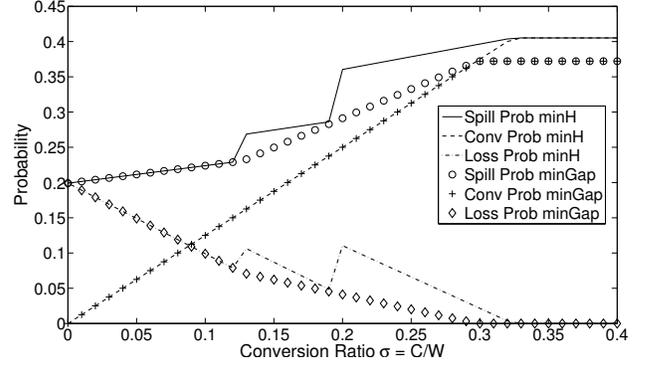
Figure 4. Comparison of policies for a switch with  $N = 3$ ,  $\rho = 0.8$ ,  $D = 10$ , geometric arrivals and packet size equal to  $\{8, 12\}$
