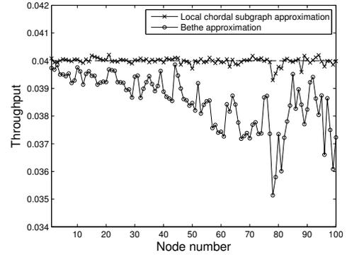
Figure 3: Throughputs of *local chordal subgraph* and *Bethe approximation* for the conflict graph in Figure 2 (by simulation) when the target throughput  $\theta_i = 0.04$  for all  $i$ .
